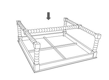
attach the bottom(C) on the legs that have been installed, after attaching fasten the top legs(B)
