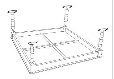
Place the Top **(A)** on the floor, attach the top legs **(B)** to the mounting holes on the top, make sure the installation is not tilted (at this step, don't tighten the top legs completely)
