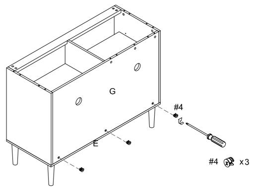
Step 12. Attach left top panel (part A) to left panel (part C) and back panel (part G) using wood dowels (part #5), cam locks (part #4) and phillips head screwdriver. NOTE: Cam locks must rotate full 180°. See pictured insert.
