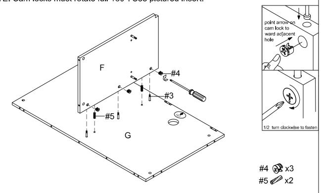
Step 6. Attach fixed shelf (part J) to dividing panel (part F) using wood dowels (part #5), cam locks (part #4) and phillips head screwdriver as shown.
