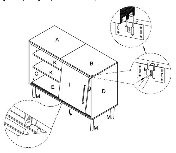
Step 16. Press the upper door pins on left door panel (part H) up.
