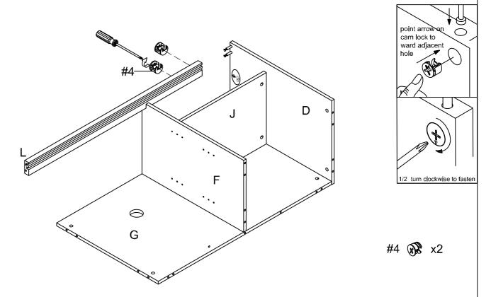
Step 9. Attach left panel (part C) to top rail (part L) and back panel (part G) using wood dowels (part #5), cam locks (part #4) and phillips head screwdriver. NOTE: Cam locks must rotate full 180°. See pictured insert.
