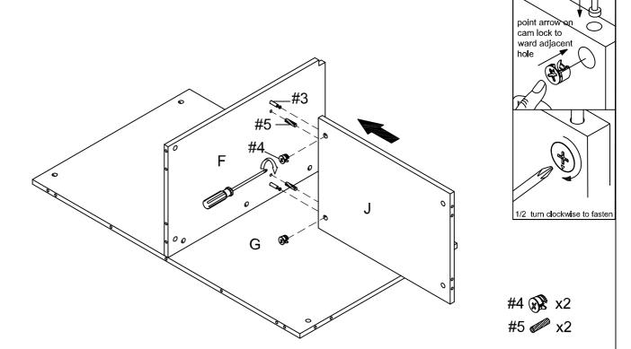
Step 7. Attach right panel (part D) to back panel (part G) and fixed shelf (part J) using wood dowels (part #5), cam locks (part #4) and phillips head screwdriver.
