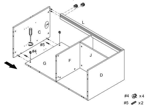
Step 10. Attach bottom panel (part E) to assembled unit (parts C, D, F & G) using wood dowels (part #5), cam locks (part #4) and phillips head screwdriver. NOTE: Cam locks must rotate full 180°. See pictured insert.
