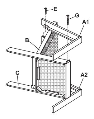
Turn the Chair over and attach right side frame (A1) into back support (B) and seat (C). Secure with 3 1/4" bolts (G) and 1" bolts (E) as shown.
