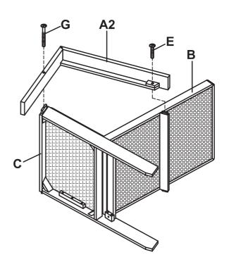
Next, attach left side frame (A2) into pre-assembled. Secure with 3 1/4" bolts (G) to Seat (C) and 1" bolts (E) to Back support (B) as shown. Do not fully tighten all bolts yet.
