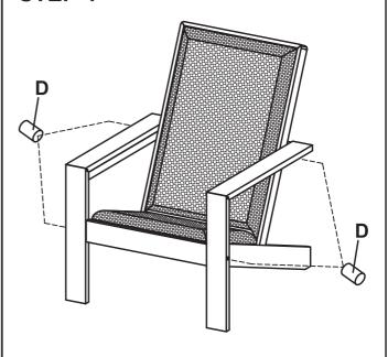
Make sure all parts are correctly connected and tighten all bolts using screwdriver .
