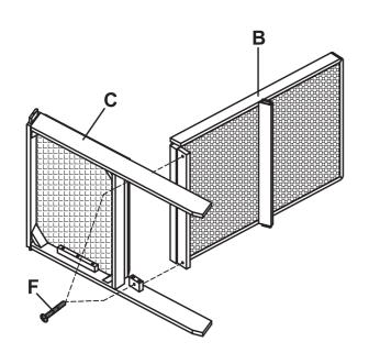
Attach back support (B) into seat (C). secure with 1 1/4" bolts (F)
