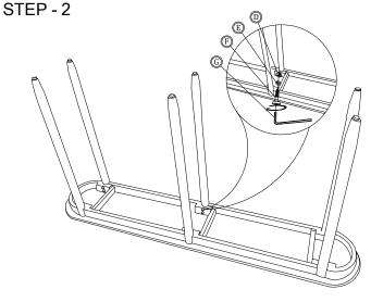
Attach to the 6 legs (B), adjust to the mount on the top(A), then attach the JCBC M6 x 40 (F) with washer (D)and spring washer (E), tighten with allen key (G)
