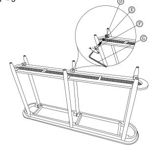
Install the shelf (C) on the legs according to the hole in the leg, Install the JCBC M6 x 40 (F) along with the washer (D) and spring washer (E), (tighten with an allen key (G))
