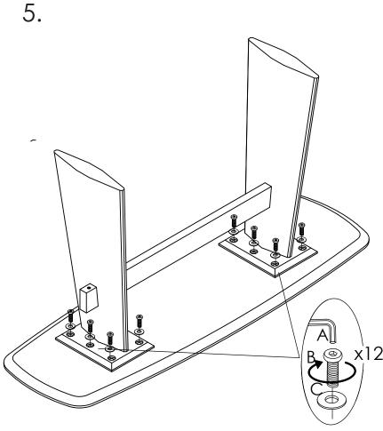
Use the wrench (A) to tighten the screws all the way.
