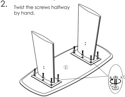
During assembly, hand tighten screws only. When the screws are in place, tighten completely.
