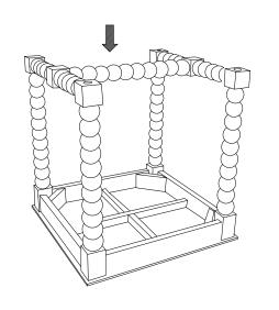
attach the bottom **(C)** on the legs that have been installed, after attaching fasten the top legs **(B)**
