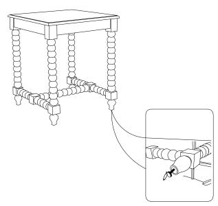
Leveller are provided at the bottom to the balance on uneven surface
