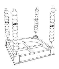
Place the Top **(A)** on the floor, attach the top legs **(B)** to the mounting holes on the top, make sure the installation is not tilted (at this step, don't tighten the top legs completely)
