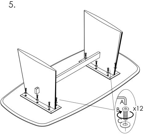
Use the wrench (A) to tighten the screws all the way.
