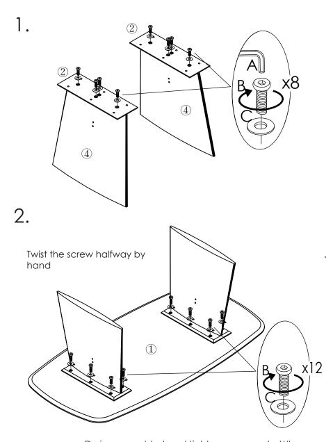
During assembly, hand tighten screws only. When the screws are in place, tighten completely.
