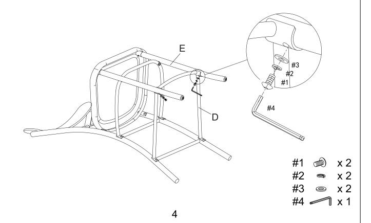
Step 5. Secure stretcher (part D) to back (part A) using bolts (part #1), spring washers (part #2), flat washers (part #3) and allen wrench (part #4).
