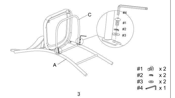
Step 3.Attach front legs (part E) to seat (part B) and top stretcher (part C) using bolts (part #1), spring washers (part #2), flat washers (part #3) and allen wrench (part #4).
