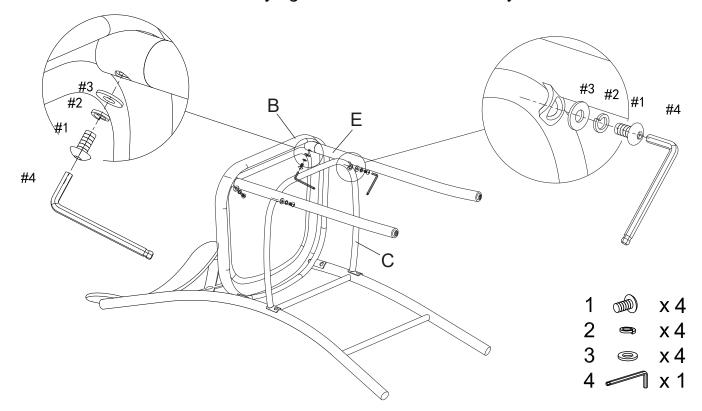
Step 4. Attach stretcher (part D) to front legs (part E) and back (part A), using bolts (part #1), spring washers (part #2), flat washers (part #3) and allen wrench (part #4).
