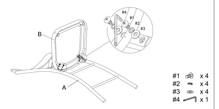
Step 2. Attach top stretcher (part C) to back (part A) using bolts (part #1), spring washers (part #2), flat washers (part #3) and allen wrench (part #4).
