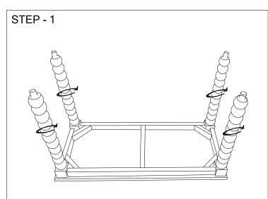
Place the Top **(A)** on the floor, attach the top legs **(B)** to the mounting holes on the top, make sure the installation is not tilted (at this step, don't tighten the top legs completely)
