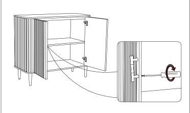
Install the handle on the outside of the door, then tie it with a screw and tighten it with a screwdriver
