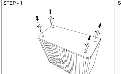
place the cabinet on the floor upside down and attach to the 4 legs (A)
