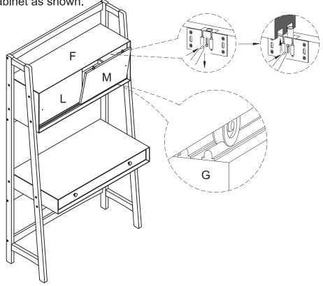
Step 12. Attach knobs (part #6) to left door panel of cabinet (part L) and right door panel of cabinet (part M) using round head bolts (part #7) and phillips head screwdriver.
