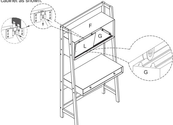
Step 11. Put the right door panel of cabinet (part M) on the outer runner of bottom panel of cabinet (part G). Press the upper door pins on right door panel of cabinet (part M) down and hold the pins next to the outer groove of top panel of cabinet (part F) then release to make sure the right door panel of cabinet (part M) is attached to pre-assembled cabinet as shown.
